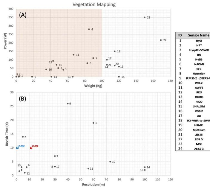
**Fig. 1.** (A) Scatter-plot of weight and power values of the satellite sensors supporting vegetation mapping applications. The red area encloses values fulfilling CLOSE mission requirements. (B) Scatter-plot of spatial resolution and revisit time of sensors lying within the red area in plot A. Number labels correspond to sensors according to the table on the right side.
