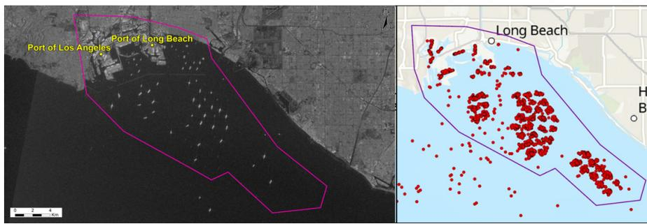
**Fig 1.** Ships waiting at the port of Los Angeles/Long Beach on Sentinel 1 image (Sentinel-1B (2021) (acquired on 25/03/2021 at 13:52 UTC, GSD 10.0 m) provided under COPERNICUS by the European Union and ESA)(left) and processing on ArcGIS pro (right).
