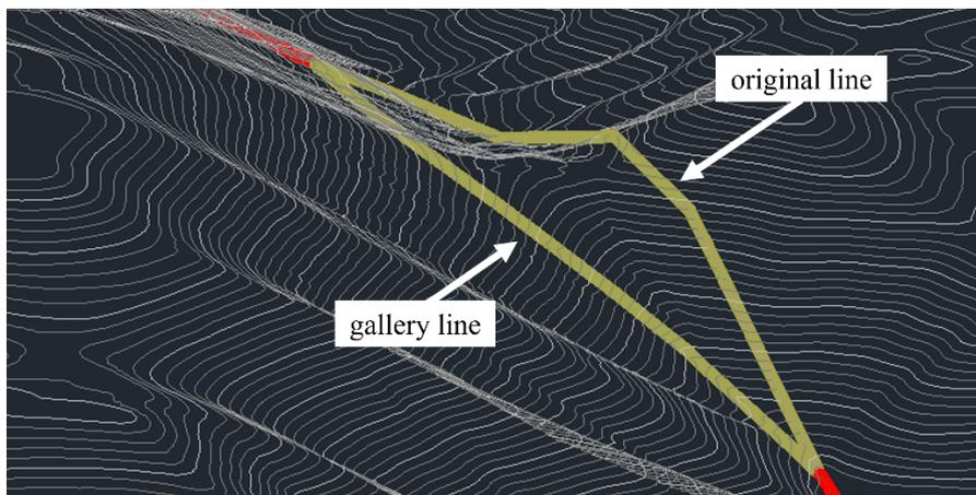
**Fig. 5.** 'Sellata' gallery (length: 1146 m; altitude: about 1120 m). The 'original line' follows DTM elevation, while 'gallery line' is the correct position.
