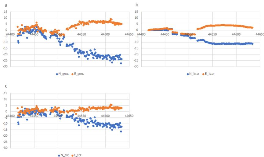
**Fig. 1.** Upper left: (a) GNSS displacements (landslide + rotations). Upper right (b): ISTAR displacements (rotations). Lower left (c): residual displacements (landslide only). In blue North direction, in orange East direction. Vertical scale is in millimeters. Time spans from June 8<sup>th</sup>, 2021, to March 13<sup>th</sup>, 2022.
