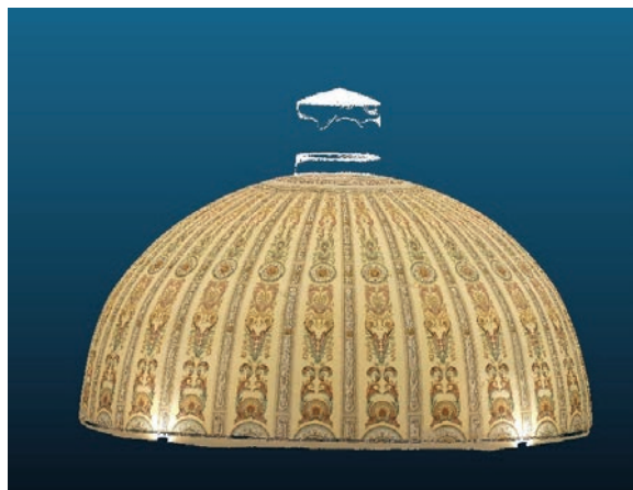
Figura 50: TLS point cloud
