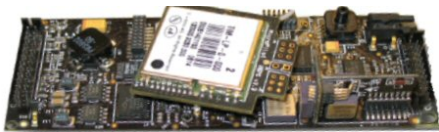
Figura 2 – Scheda autopilot MP2128 HELI .
