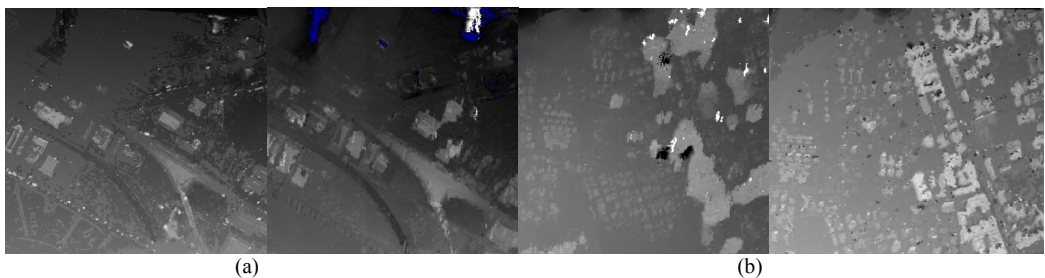
Fig. 2 – (a) SISAR DSM (left) e OrthoEngine DSM (right) di Augusta open area (b) SISAR DSM (left) e OrthoEngine DSM (right) di Augusta urban area.
